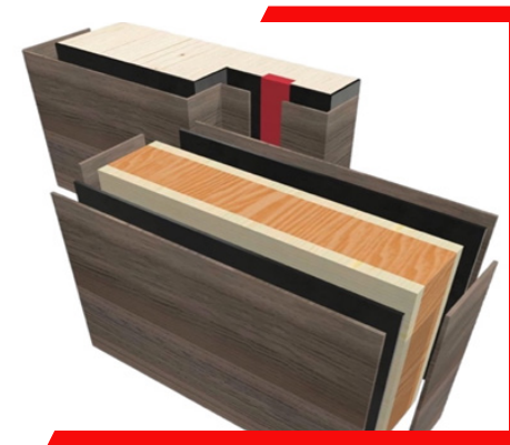
VFL as fire resistant intumescent barrier foil for doors
